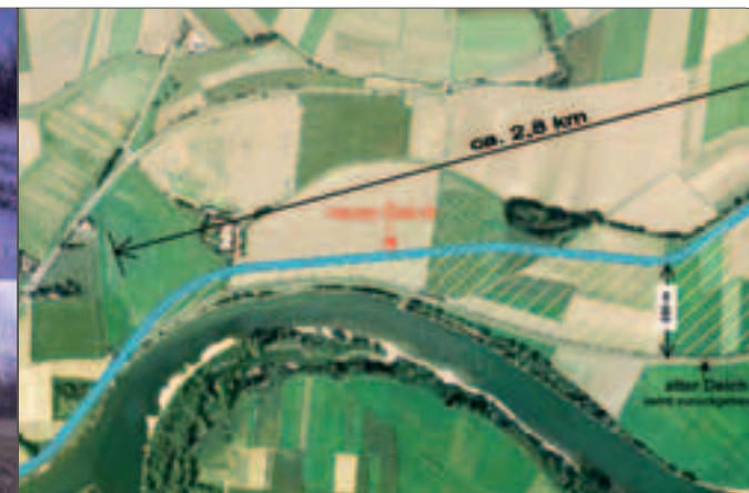
Relocation of dikes
